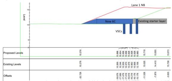
Figure 33: Section adjacent to Farm Access Underpass Extension showing zone of ground improvement
